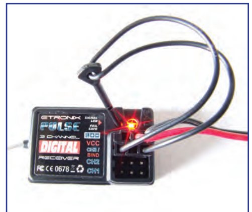
Once the 'Bind' process is complete, the throttle failsafe position can be set by pressing the button using the pointer provided.
