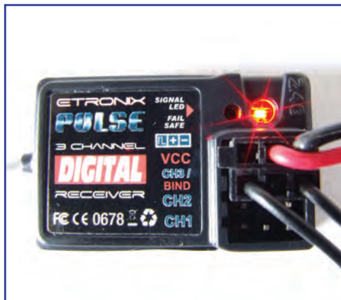
To 'Bind' the receiver to the transmitter the supplied Bind Plug should be installed channel 3/bind socket before power is applied. The red LED should begin to flash to indicate the 'Bind' process has begun, and go solid red once 'Bind' is complete. Now remove the 'Bind' plug and restart the power up procedure.
