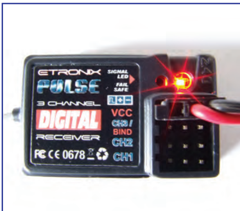
Unless a battery powered model using an ESC with BEC, a receiver pack should be plugged into the VCC socket via a suitable power switch, making sure to check for correct polarity.
